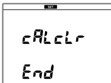
7. Press the ENTER key to return to the calibration data clear screen.
