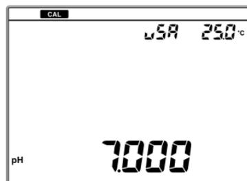
6. Check the stable indication value, and press the CAL key.
