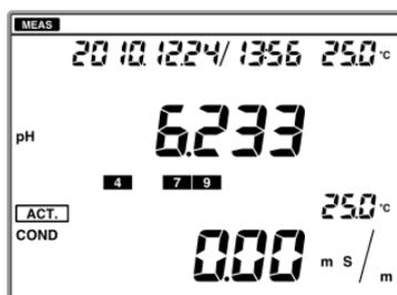
5. Press the CAL key on the measurement screen is displayed to enter the calibration screen.
