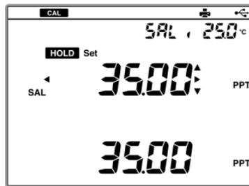
8. After the calibration is completed, press the MEAS key to return to the measurement screen.
