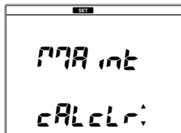
4. Press the ENTER key and the ◀ or ▶ key to select the measurement item to be deleted.
