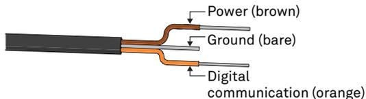
Figure 2 Pigtail wiring
