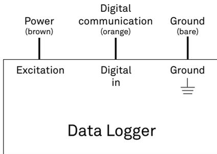
Figure 3 Wiring diagram
