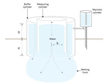
Figure 33 Cross section of a double-ring infiltrometer
