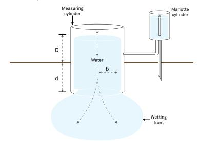
Figure 32 Cross section of a single-ring infiltrometer
