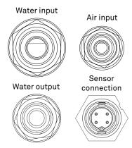
Figure 15 Control unit connections
