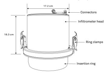
Figure 30 Infiltrometer head
