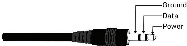
Figure 2 Stereo plug connector
