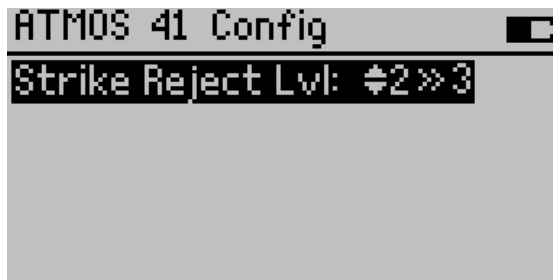
Figure 24 Adjusting the ATMOS 41 strike reject level
