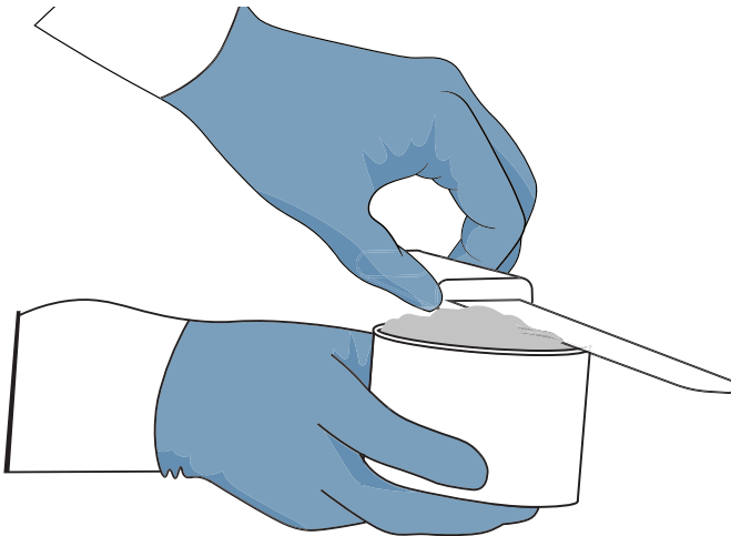
Figure 6 Cut protruding material level with edge of sample ring
