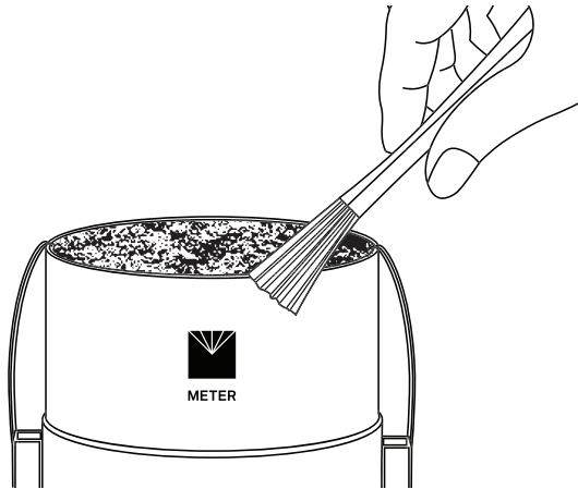
Figure 49 Fix and clean the soil sampling ring
