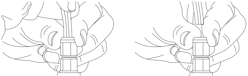
Figure 81 Removing the tube
