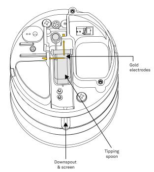
Figure 16 Downspout and screen
