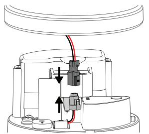
Figure 15 Connect pyranometer cable
