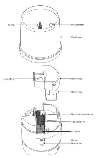
Figure 12 Rain funnel and rain gauge
