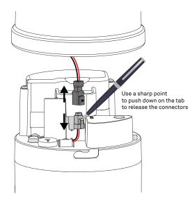
Figure 14 Disconnect pyranometer connector
