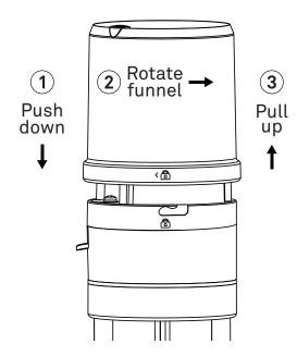
Figure 13 Removing ATMOS 41 Gen 2 rain funnel
