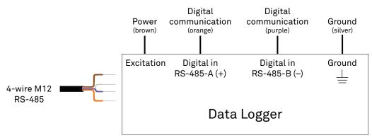
Figure 6 Four-wire M12 connector RS-485 wiring diagram
