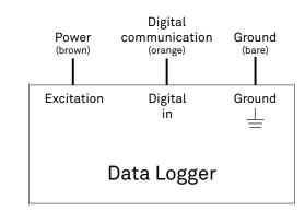
Figure 3 Three-wire SDI-12 wiring diagram
