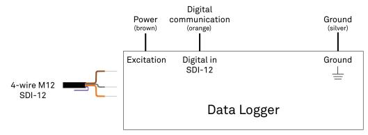
Figure 4 Four-wire M12 connector SDI-12 wiring diagram
