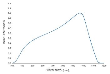
Figure 9 Spectral response estimate of Apogee silicon-cell pyranometers
