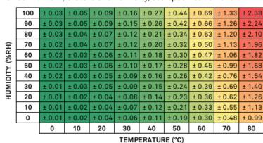
Figure 7 Vapor pressure sensor accuracy
