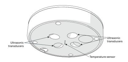
Figure 19 Temperature needle and ultrasonic transducers
