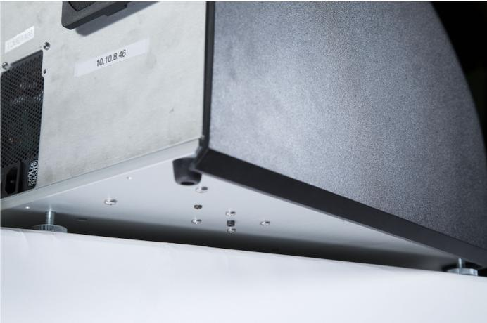
Figure 5: Locate Shipping Screw
