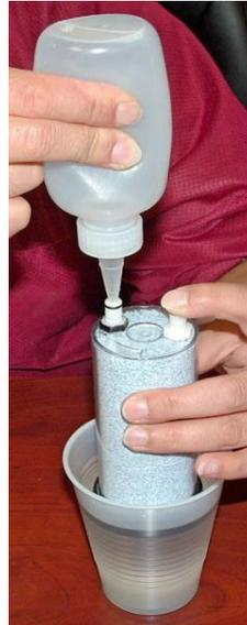
Figure 33: Checking Desiccant Cartridge for Leaks
