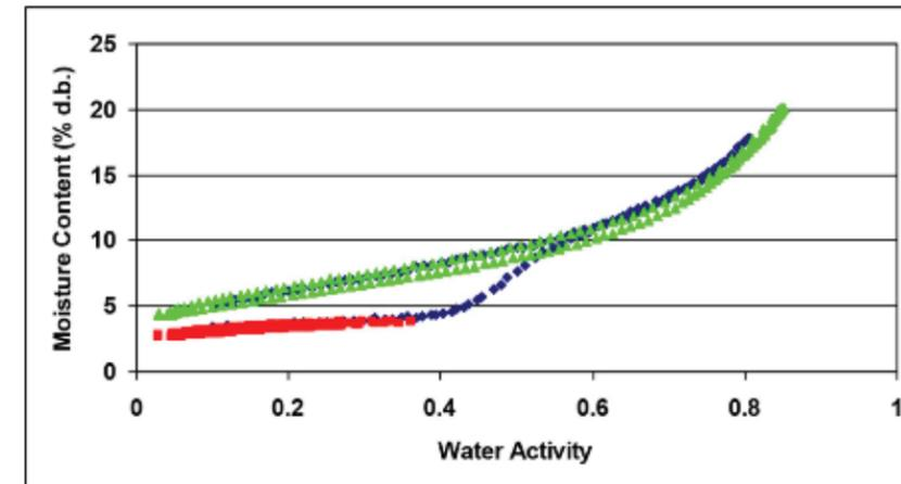
Figure 22 Spray-dried milk moisture sorption isotherms
