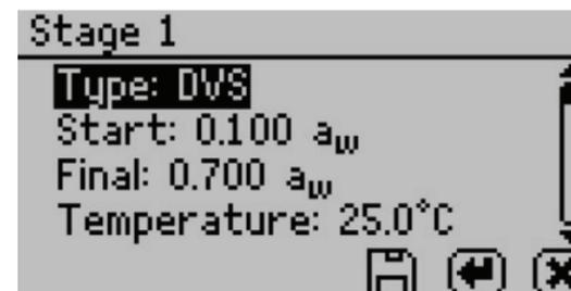
Figure 44 Edit stages DVS method
