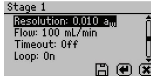
Figure 43 Edit stages DVS method
