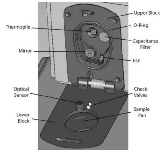
Figure 28 AQUALAB VSA sample chamber diagram
