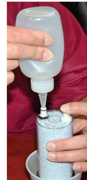
Figure 27 Checking desiccant for leaks
