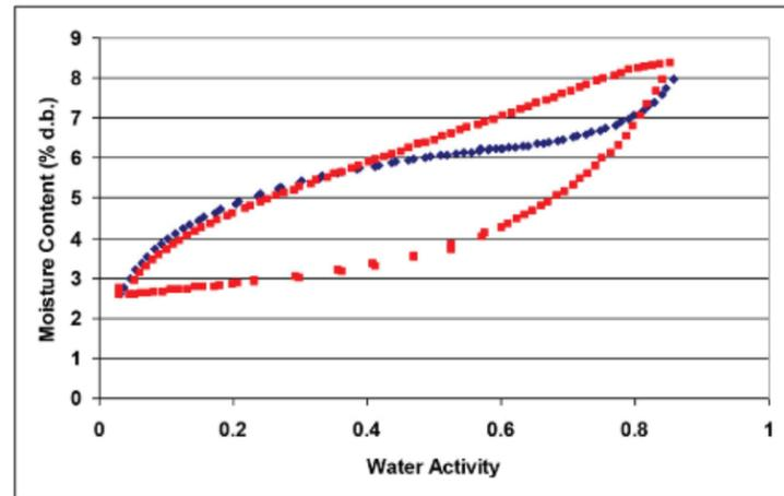
Figure 23 Working and full isotherm for wood pulp
