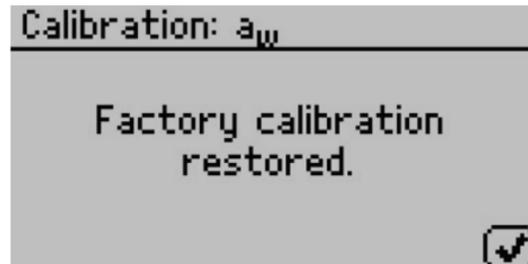
Figure 36 Confirmation that factory calibration was reset
