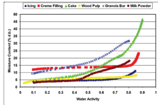
Figure 19 Moisture adsorption isotherms
