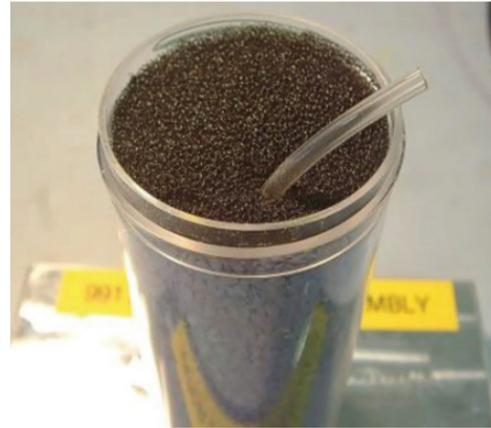
Figure 25 Desiccant cartridge foam
