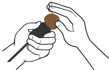
Figure 24 Pack native soil slurry on TEROS 21 sensor
