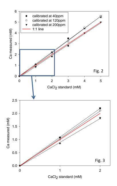
The electrode was calibrated at 40, 120 or 200 ppm (1, 3, 5 mM) and tested in a range of CaCl2 standards from 1 to 5 mM, a range expected in the xylem sap samples to be analysed.
