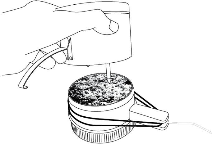
Figure 15 Assembling the HYPROP unit
