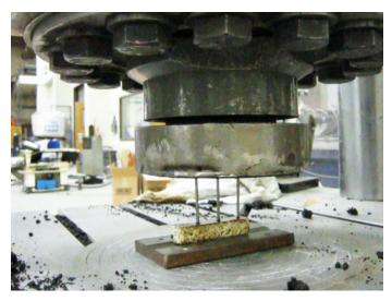
Figure 4. Sensor 1 in compression machine.
