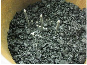
Figure 2. Sensor 1 centered in Sample 1.
