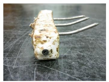
Figure 9. Sensor 1 after compression testing (vertical orientation).
