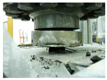
Figure 5. Sensor 2 in compression machine.
