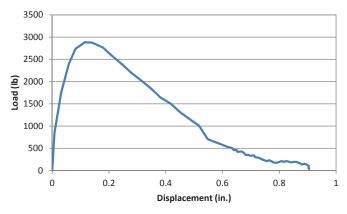
*Figure 6. Load - displacement plot for Sample 1 (vertical orientation).*
