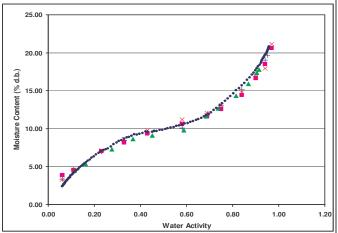
Figure 2. Corn starch working isotherms when using desiccators with saturated salts ( $\blacksquare$ ), Proximity Equilibration Cell ( $\bullet$ ), DVS instrument 1 ( $\bullet$ ), DVS instrument 2 ( $\blacktriangle$ ), and DDI ( $\times$ ) (DDI data from Decagon Devices in-house testing, data for all other methods taken from (Xin Yu, 2007)).
