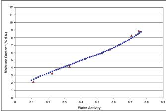
Figure 1. A comparison of adsorption isotherm curves for MCC as recorded by the COST 90 project ( $\blacktriangle$ ) and as generated by the DDI method ( $\blacksquare$ ).
