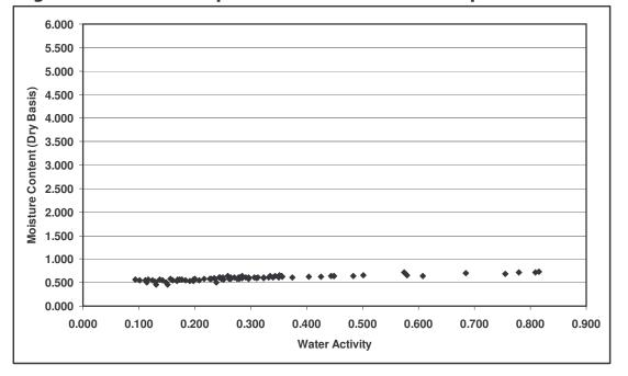
Figure 1. Moisture sorption isotherm for PVC resin pellets at 25°C.
