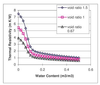
**Figure 2** Effect of density and water content on thermal resistivity of a loam soil. The void ratio 1 curve is the same as in Fig. 1. The bulk densities are 1.06 Mg/m<sup>3</sup> for void ratio of 1.5, 1.33 Mg/m<sup>3</sup> for void ratio 1, and 1.59 Mg/m<sup>3</sup> for void ratio of 0.67.
