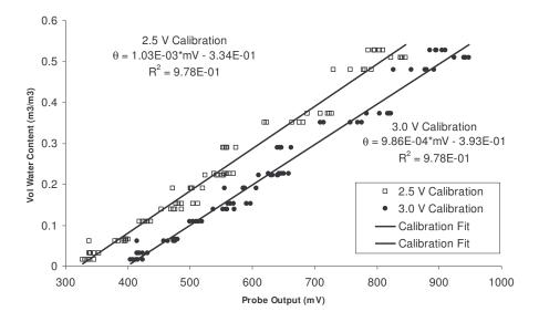
**Figure 2.** Calibration curve for EC-5 in rockwool at 2.5 V excitation and EC levels of 0.2, 1, 1.5, 1.8, and 4.2 dS/m.
