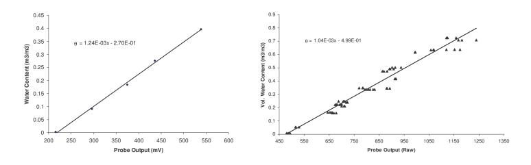
Figure 5. A single ECH<sub>2</sub>O-TE calibration in rockwool at EC levels of 0.002, 4.1, and 8.1 dS/m.
