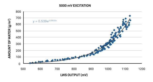
Figure 3. Amount of water on PHYTOS 31 surface as a function of PHYTOS 31 mV output when excited at 5000 mV
