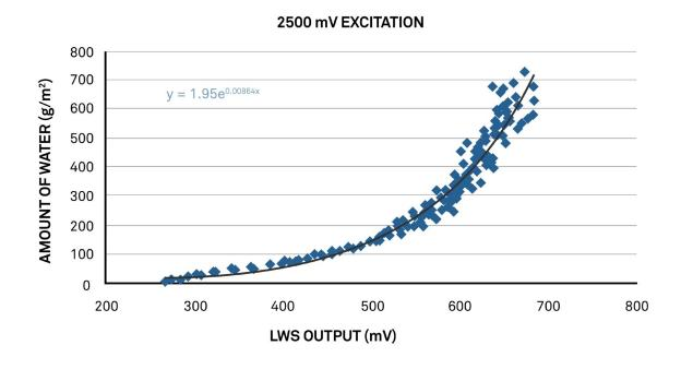
Figure 2. Amount of water on PHYTOS 31 surface as a function of PHYTOS 31 mV output when excited at 2500 mV. This relationship can be used with Campbell Scientific of other third-party data acquisition systems that excite the PHYTOS 31 at 2500 mV.
