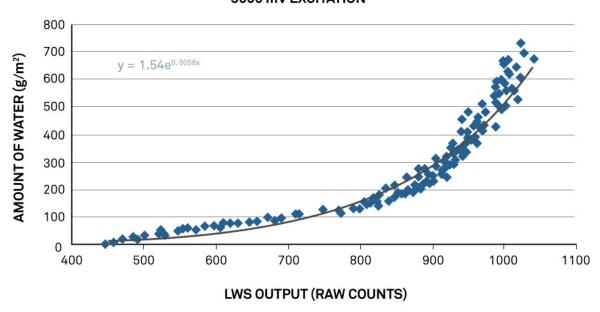
Figure 1. Amount of water on PHYTOS 31 surface as a function of PHYTOS 31 raw counts measured with METER EM50 series data logger
