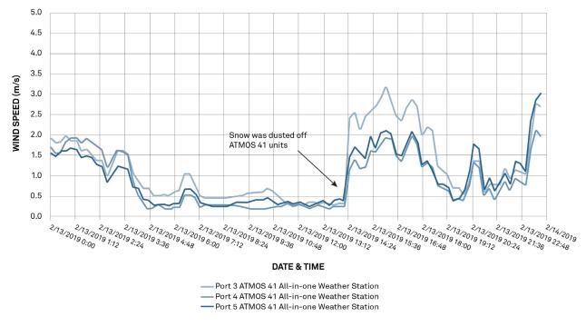
Figure 3. ATMOS 41 wind speed data
