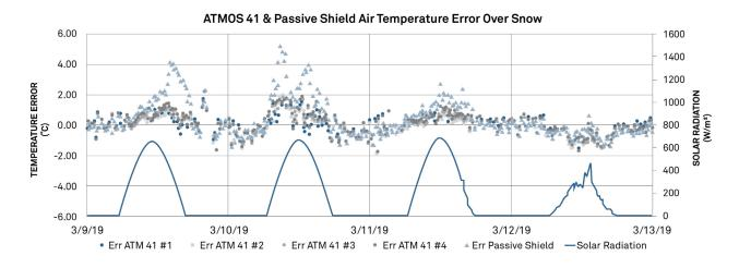
Figure 6. ATMOS 41 and non-aspirated radiation shield air temperature error over snow. March 9 and 10 had low wind speeds, giving a worst-case air temperature accuracy.
