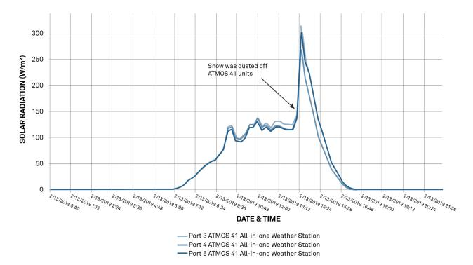
Figure 2. Atmos 41 solar radiation data
