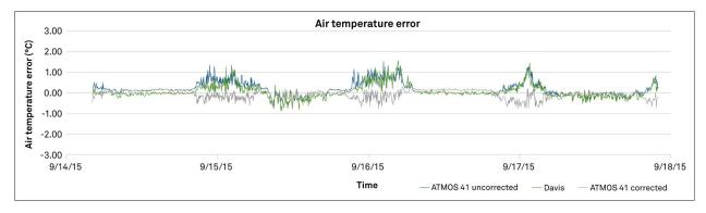
Figure 1. Environmental conditions and air temperature error (T<sub>measured</sub> – T<sub>TS-100</sub>) for the two air temperature sensors under evaluation
