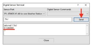
Figure 26. ?Xc! command verified CAL Factor, response
