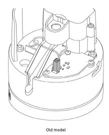
Figure 1. Rain funnel and pyronometer connector
