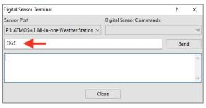
Figure 25. ?Xc! command to verify CAL Factor, entered
