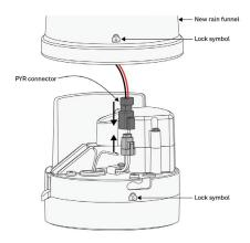
Figure 5. Pyranometer cable connector
