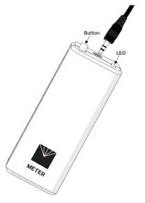
Figure 9. Plug sensor stereo connector into ZSC
