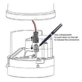
Figure 2. Removing ATMOS 41 rain funnel
