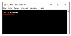
Figure 31. Enter CAL Factor value for replacement funnel
