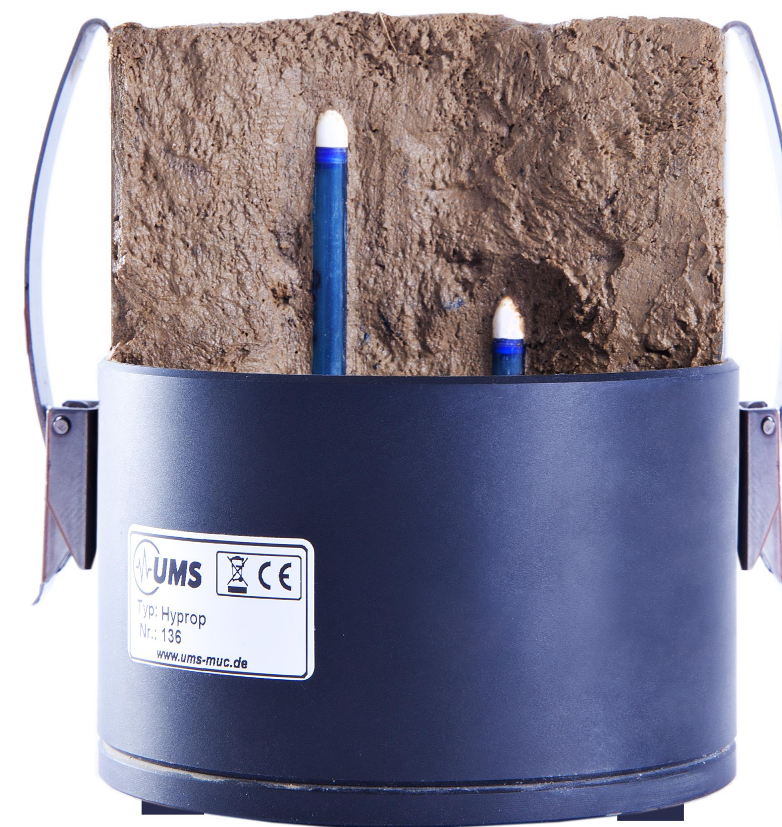
Figure 1: Cutout of the HyProp showing placement of the two tensiometers in the soil.
