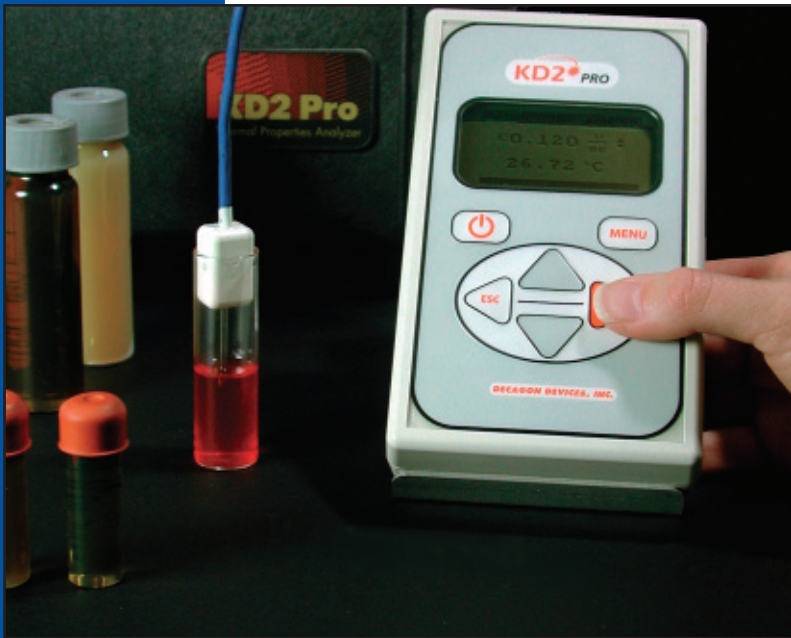
■ Thermal properties of oil samples being measured with KD2 Pro.
