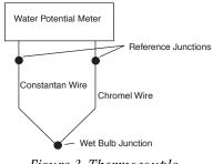
Figure 3: Thermocouple
