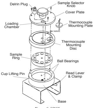
thermocouple is mounted on the underside.
