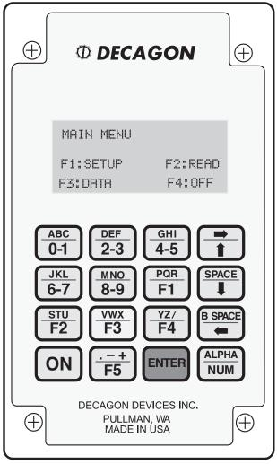
Figure 2: Microcontroller Keypad
