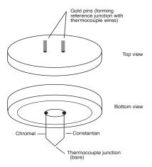
*Figure 7: Peltier thermocouple*
