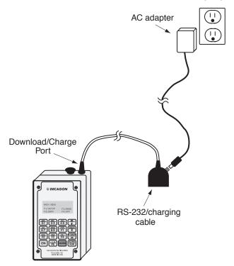
Figure 4: Recharge setup
