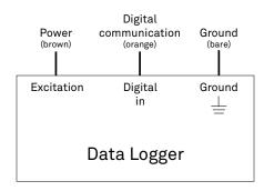
Figure 3 Wiring diagram
