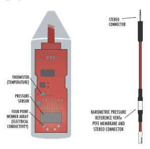
Figure 4 HYDROS 21 component diagram
