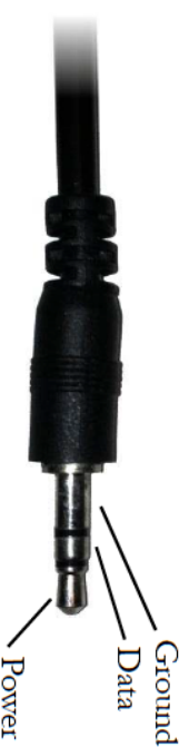
Figure 5: 3.5 mm Stereo Plug Wiring
