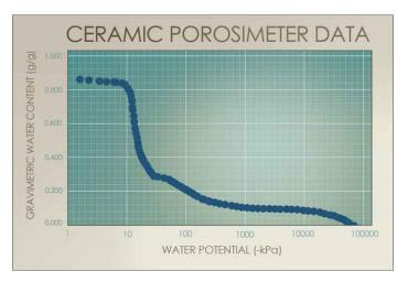
Figure 2: Moisture characteristic curve derived from mercury porosimeter data for MPS-2 and MPS-6 ceramic
