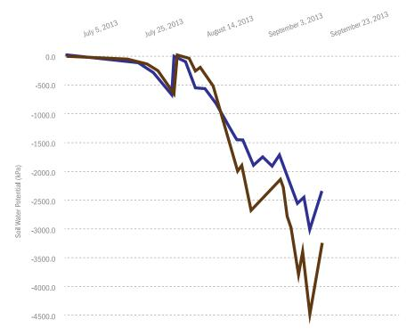
Figure 4: Time series MPS water potential data collected at 20 cm under a dry oak forest in Switzerland. Note the range extends well beyond permanent wilting point.<sup>3</sup>
