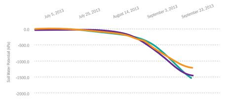
Figure 3: Time series MPS water potential data collected at 80 cm depth under a Beech forest in Switzerland. Note the excellent sensor agreement down to permanent wilting point (-1,500 KPa).<sup>3</sup>
