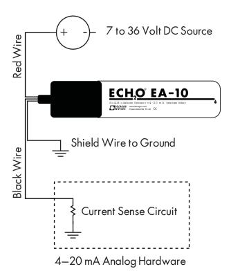
The red wire is connected to the positive terminal and the black wire is the return for the negative terminal. The shield (bare wire) can be connected to a shield terminal, if available, or left open. The probe is electri-
