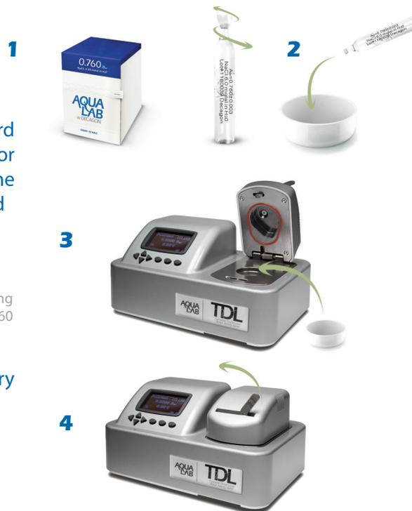
Important: The bag of lids is to cover samples to prevent moisture loss or gain if you do not immediately test samples. Do not place a sample cup with a lid into the chamber.
