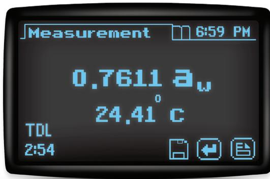
The final reading will be displayed after the instrument 'beeps' and the 'Save' icon appears. The temperature displayed is the sample temperature. Use a new cup for each sample.
