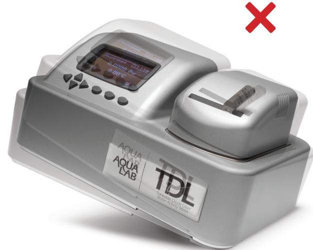
Important: Avoid tipping or moving the instrument with a sample in the chamber. This may contaminate the sensors.
