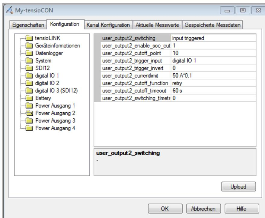
**Figure 25: tensioCON configuration register**
