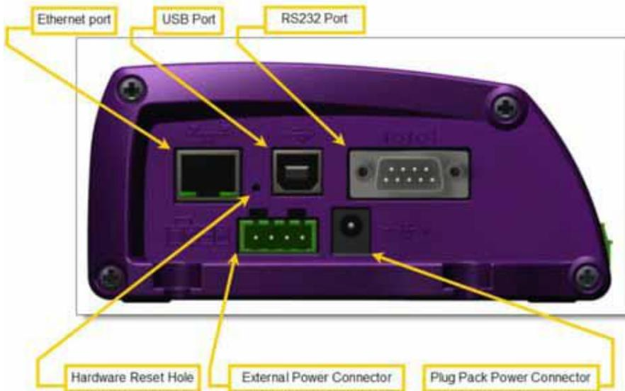
Figure 41: connections and reset hole
