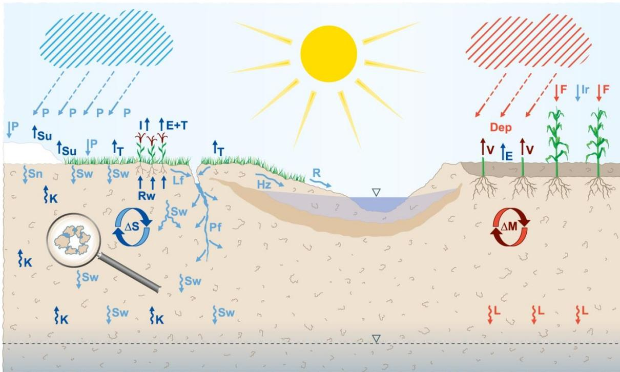
Figure 37: water balance parameters
