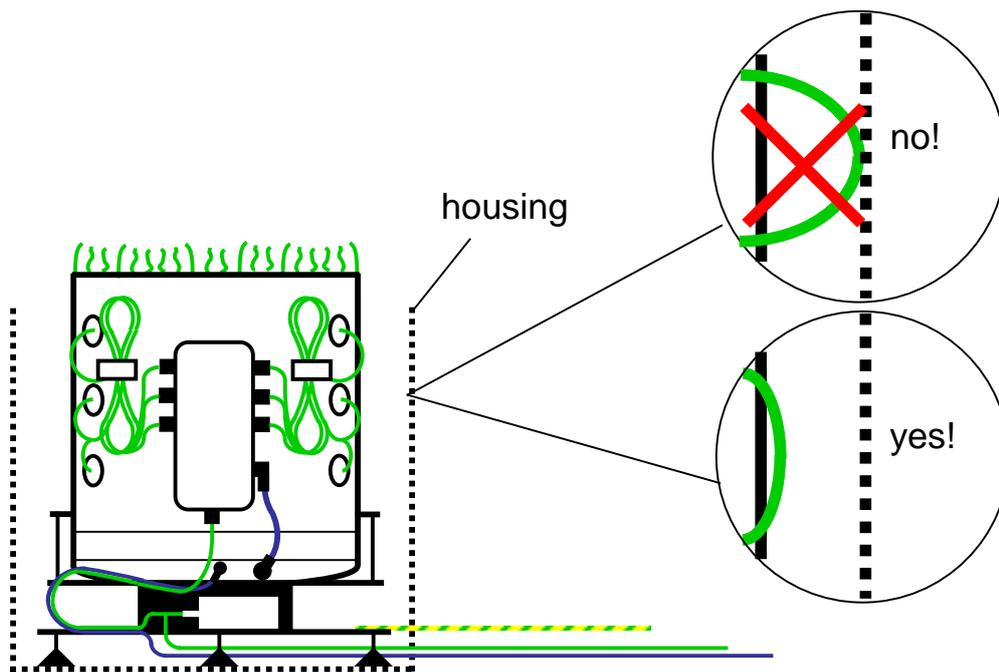
Figure 27: adjusting and centering the Lysimeter
