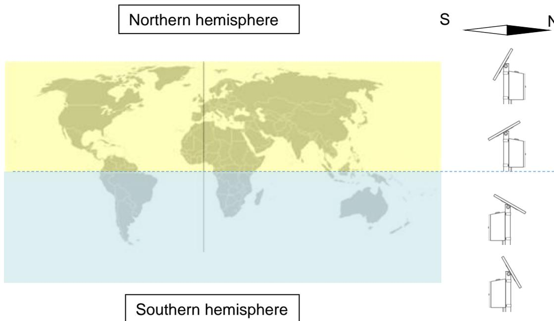
Figure 28: orientation and angle of the solar panel depending on the location
