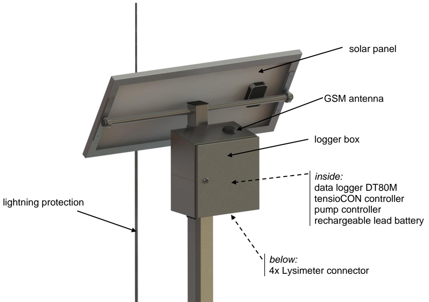
Figure 4: logger box and components
