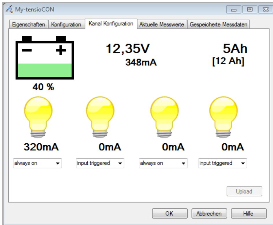
Figure 26: tensioCON battery state
