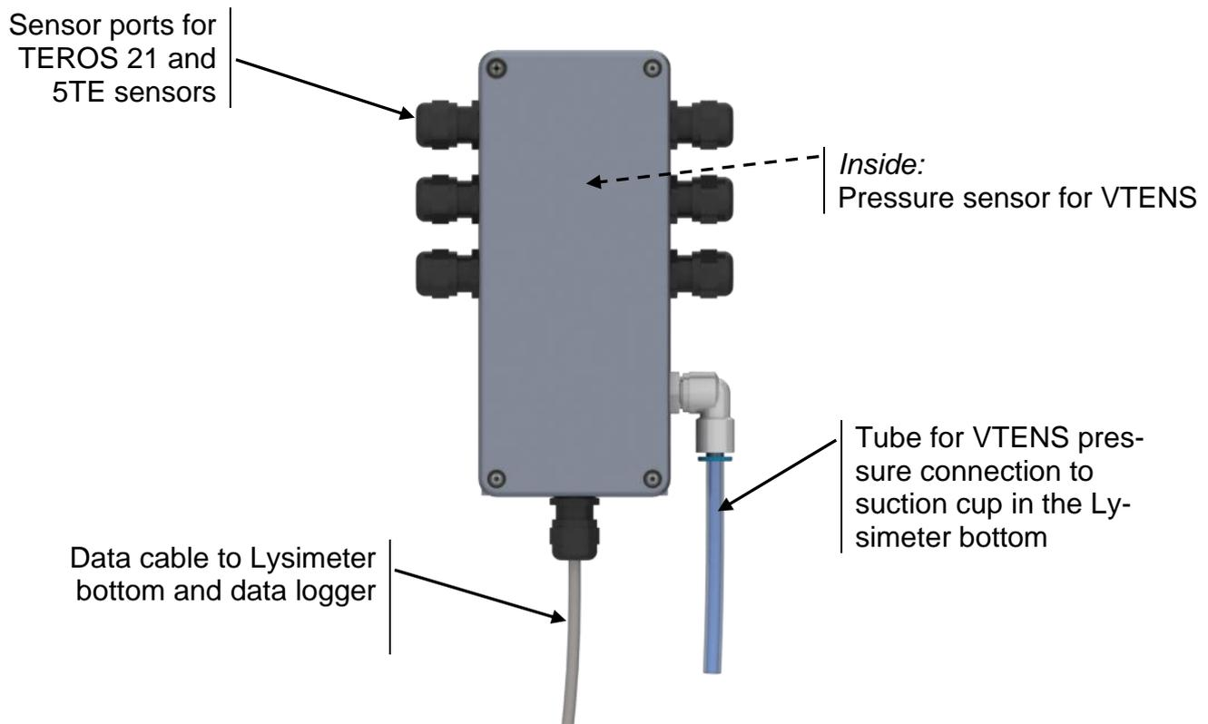
Figure 12: Lysimeter sensor distribution box
