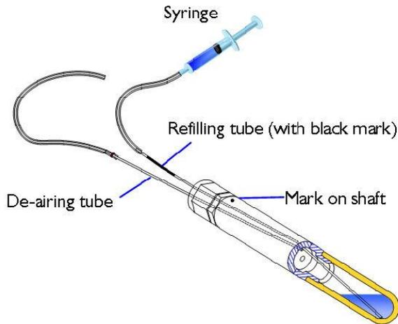
**Figure 32: downwardly installation – the marked pipe is the refilling tube, the un-marked pipe the exhaust pipe**
