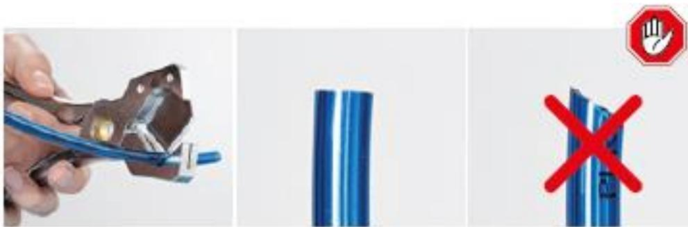
**Figure 29: cutting the tubes correctly**
