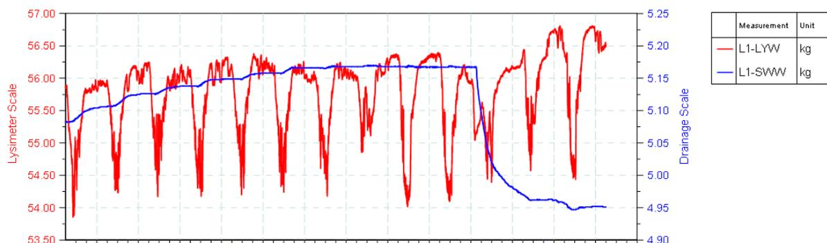
Figure 39: mechanical contact leads to temperature dependent fluctuations
