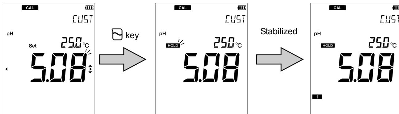
6. Perform the 2nd point calibration. As with the step 2., wash the pH electrode and immerse it in the 2nd standard solution. As with the step 4., immerse at least 3 cm from the tip of the pH electrode.
