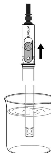
3. Immerse at least 3 cm from the tip of the pH electrode in the sample solution.
