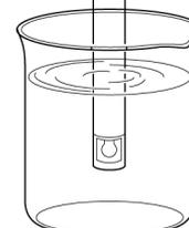
5. Check that the pH value is stable while the pH electrode is immersed in the standard solution, then press the
