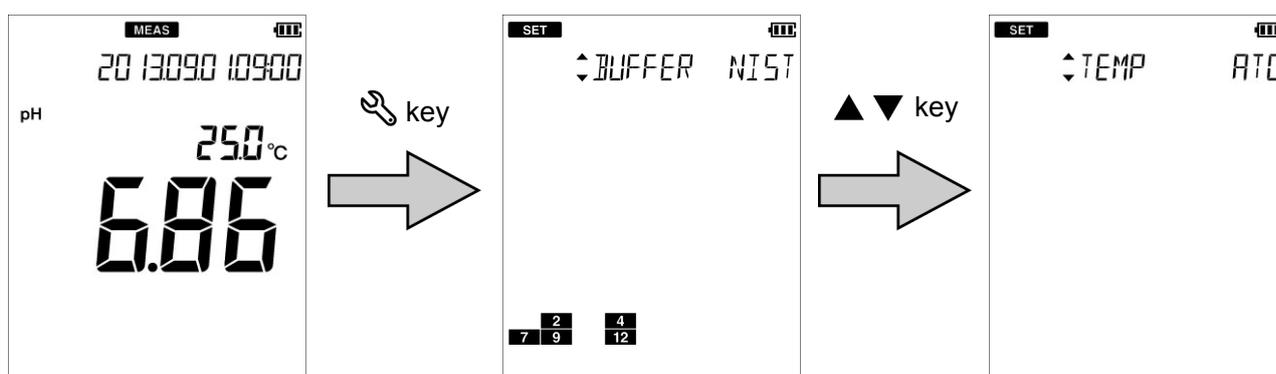
3. Press the ◀▶ keys to select the "ATC" (automatic temperature compensation) or the "MTC" (manual temperature compensation) and then press the ● key.
