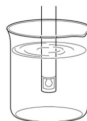
7. Press the
