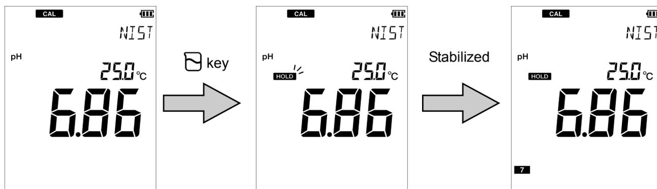
6. Perform the 2nd point calibration. As with the step 2., wash the pH electrode and immerse it in the pH 4 standard solution. As with the step 4., immerse at least 3 cm from the tip of the pH electrode.
