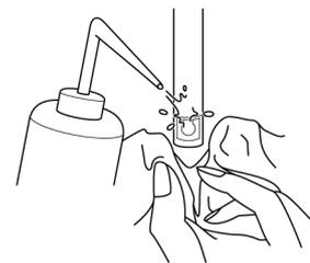
2. Open the internal solution filler port of the pH electrode.
