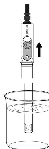
3. Immerse at least 3 cm from the tip of the pH electrode in the pH 7 standard solution.
