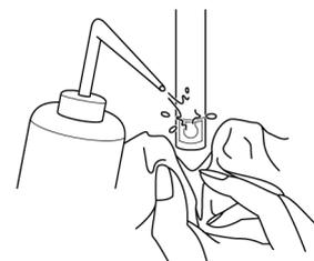
2. Open the internal solution filler port of the pH electrode.
