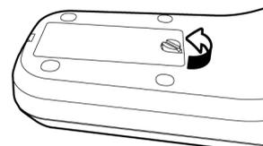
2. Remove the battery cover and set the batteries inside.
