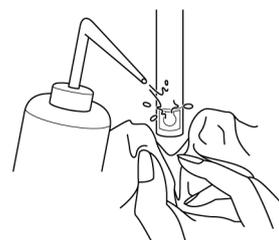
3. Open the internal solution filler port of the pH electrode.
