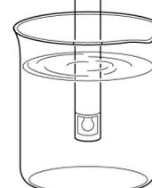
5. Check that the pH value is stable while the pH electrode is immersed in the standard solution, then press the
