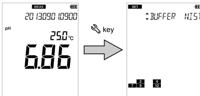
3. Press the ◀▶ keys to select "NIST", "USA", or "CUST" according to the standard solution to be used and then press the ● key.
