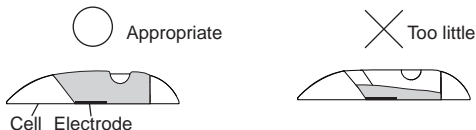
Cross-section of the measurement cell
