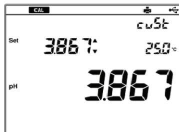
5. Press the ◀ or ▶ key to select digit and press the ▲ or ▼ key to change value, to set the value of the desired standard solution.
