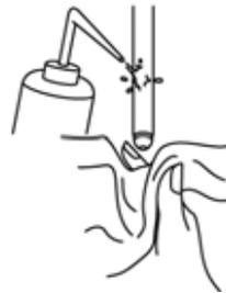
6. If the inside of the protective cap is dry, wash the inside with pure water (deionized). After shaking out the water, fill the cap with enough pure water (deionized) to soak the sponge.
