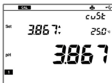
The **1** mark, which means that the first point calibration is completed, is displayed on the screen.
