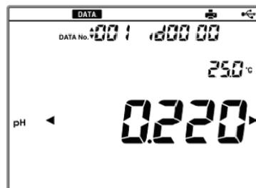
4. Press the ◀ or ▶ key to switch between date display and DATA No/ID No. display. Press the ▲ or ▼ key to search past data.
