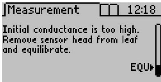
Figure 8 Warning screen for high initial conductance
