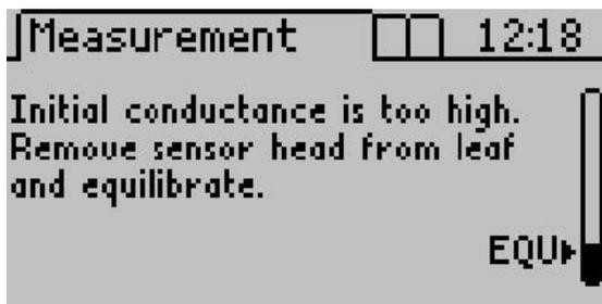
Figure 8 Warning screen for high initial conductance
