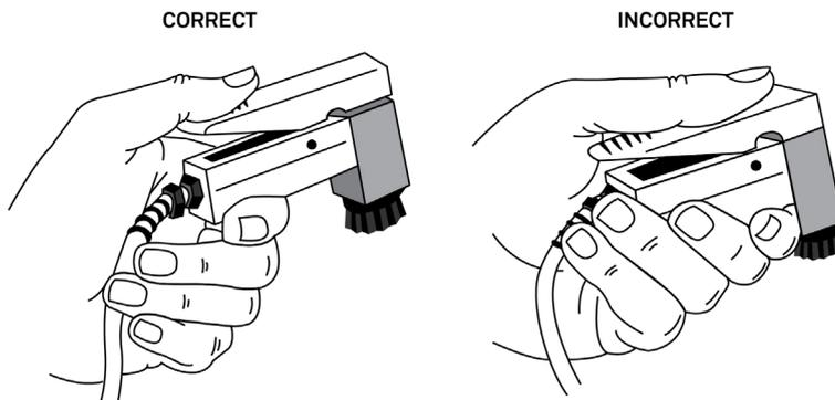
Figure 43 Holding the sensor head
