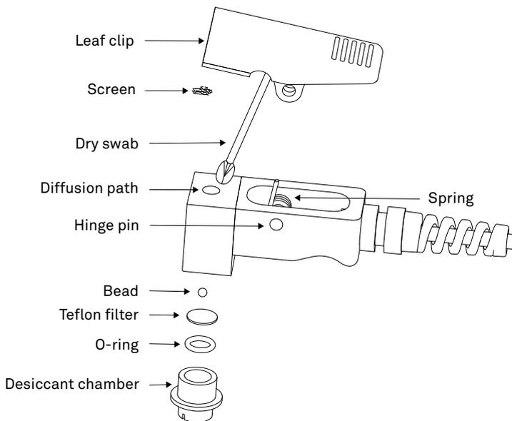
**Figure 55 Thorough cleaning of the diffusion path**
