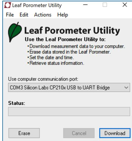
Figure 19 Leaf Porometer Utility main window
