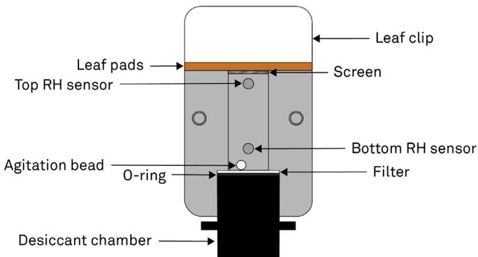
Figure 26 Sensor head internal components
