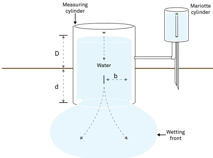
Figure 32 Cross section of a single-ring infiltrometer
