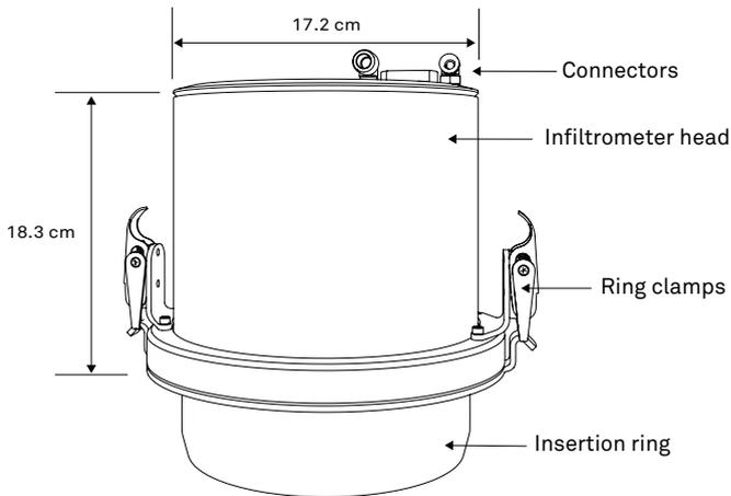
Figure 30 Infiltrimeter head
