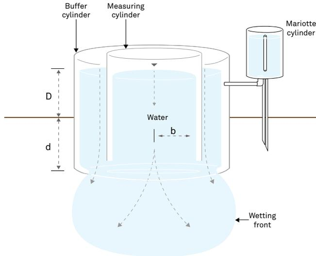
Figure 33 Cross section of a double-ring infiltrometer
