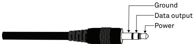
Figure 1 3.5-mm stereo plug connector wiring
