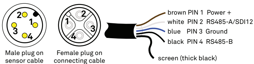
Figure 6 4-pin M12 plug wiring
