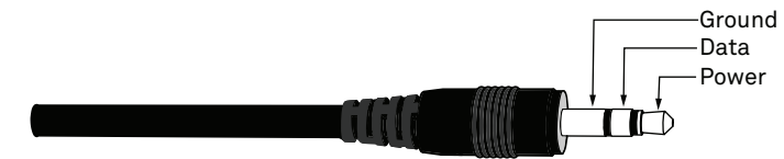
Figure 1 3.5-mm stereo plug connector wiring
