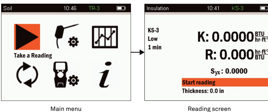
**Figure 4** Navigating to the Take a Reading screen
