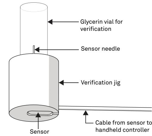
**Figure 28** Verification holder for single-needle sensors
