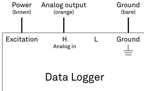
Figure 3 Wiring diagram
