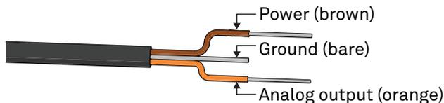
Figure 2 Pigtail wiring
