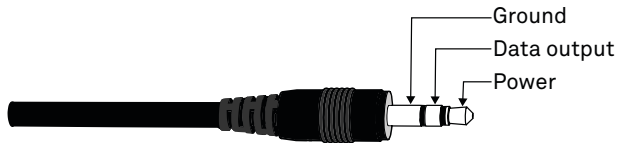
Figure 2 3.5-mm stereo plug connector wiring
