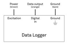
Figure 4 Wiring diagram
