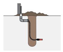
Figure 1 Example of 5TM proper installation
