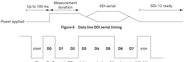
Figure 7 Example DDI serial transmission of the character 9 (0x39)
