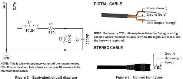
Figure 2 Equivalent circuit diagram
