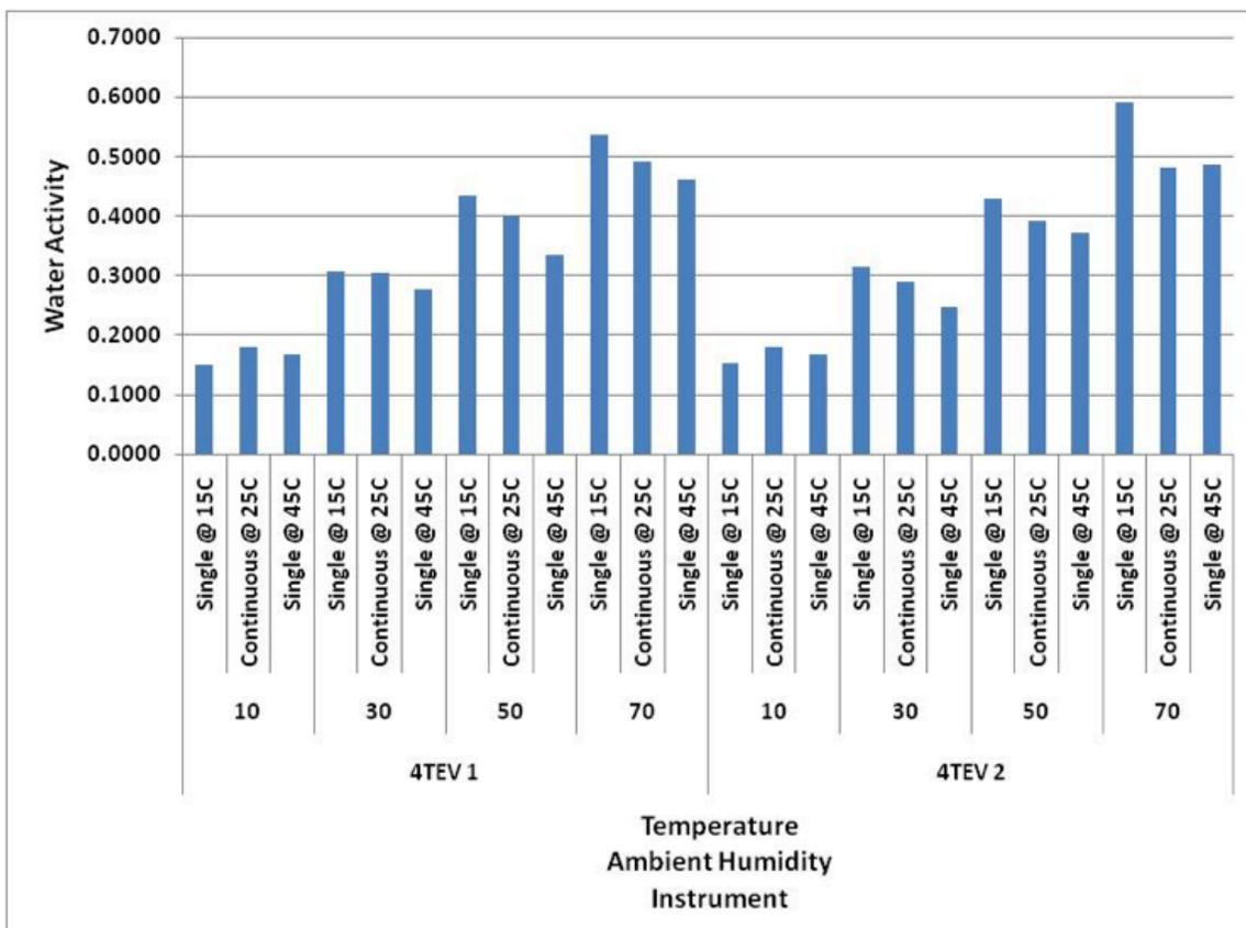
**Figure 5. Average water activity values for 2 AquaLab Series 4TEV instrument at 4 different ambient humidities and 3 different temperatures.**
