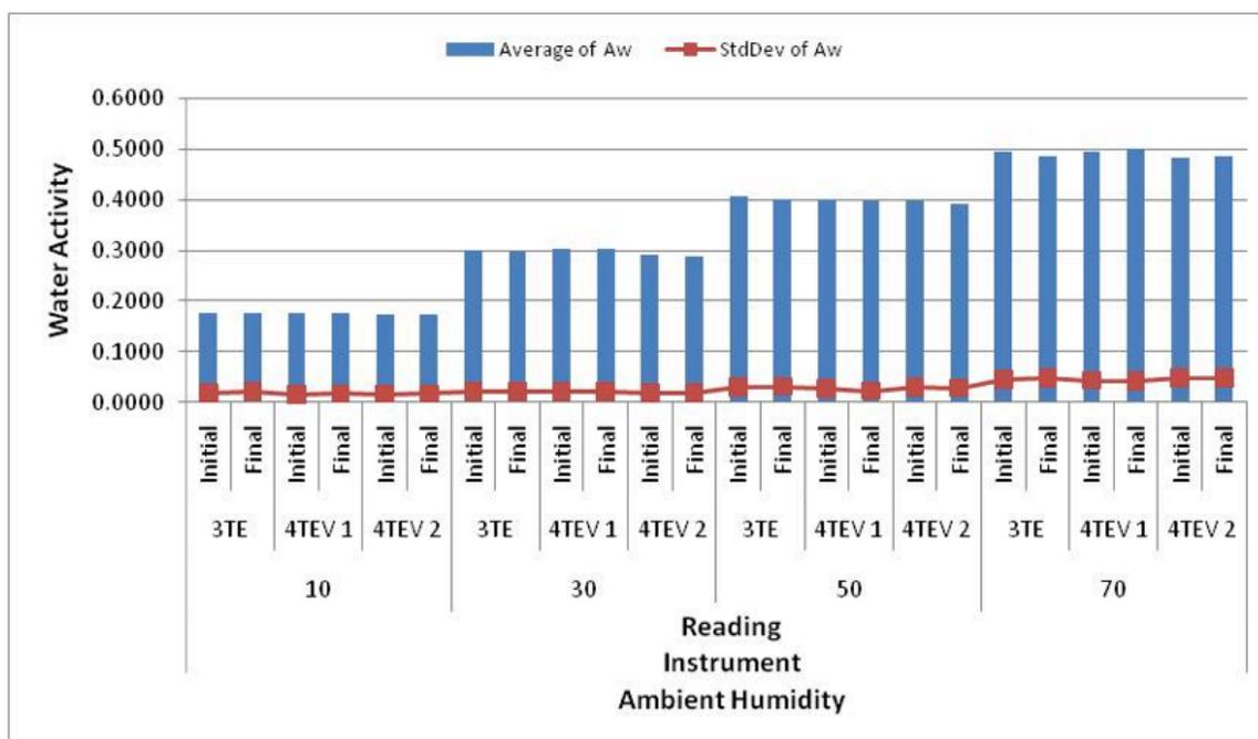
**Figure 1. Average water activities and standard deviations for 5 different water activity instruments at 4 different ambient humidities. A comparison of the initial and final reading for the dewpoint instruments is also provided.**
