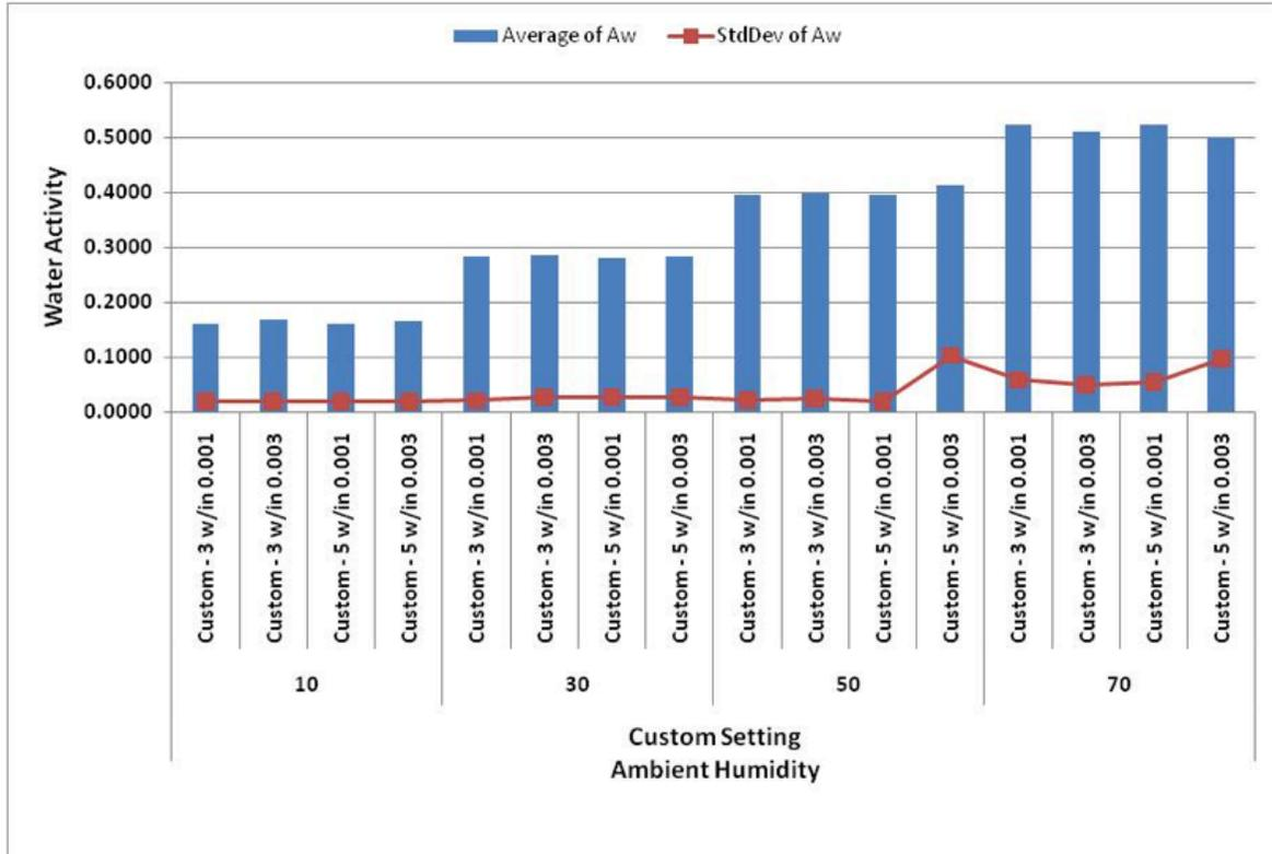
**Figure 4. Average water activity values and standard deviations for an AquaLab Series 4TEV instrument at 3 different ambient humidities when using 4 different custom mode settings.**
