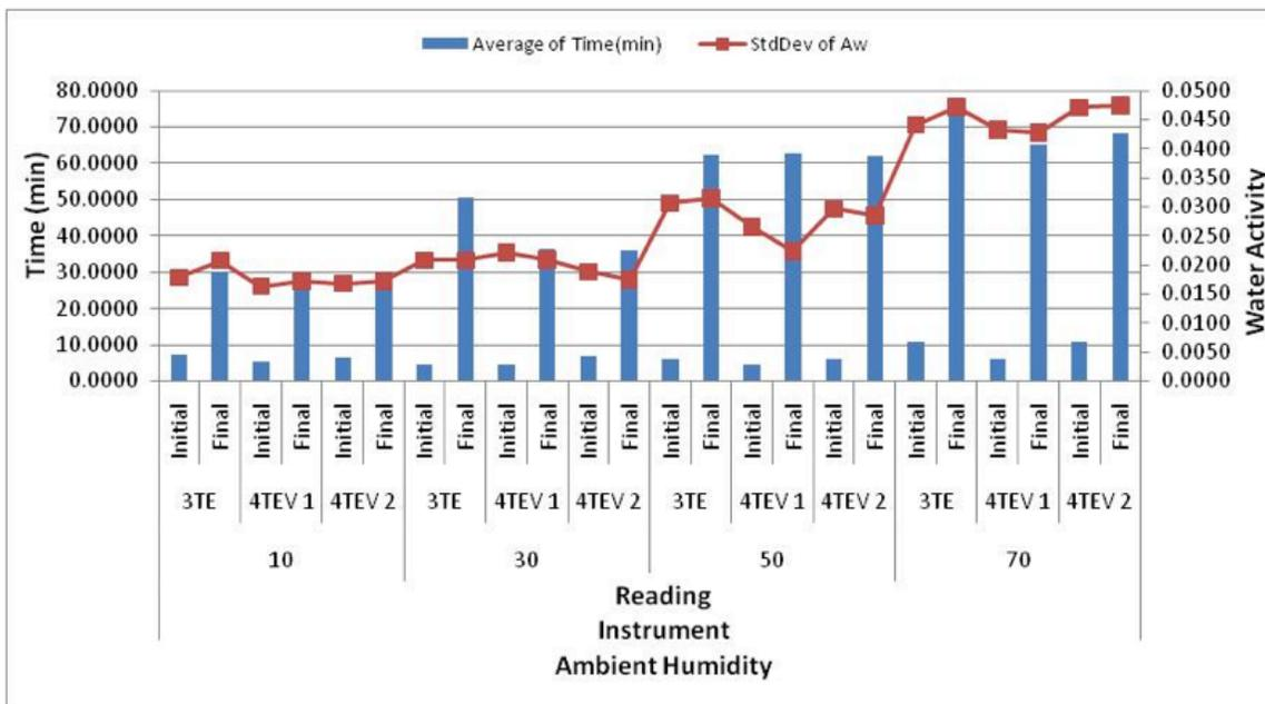
**Figure 2. Average test times and standard deviations of final and initial readings of 5 different water activity instruments at 10%, 30%, 50%, and 70% relative humidity.**
